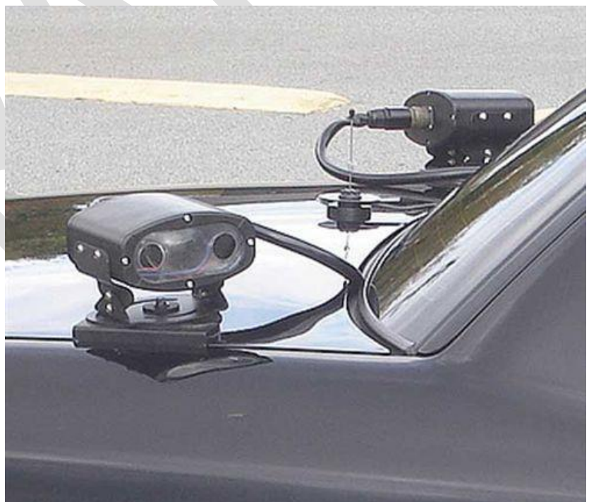
Photo 1 - Sample LPR Vehicle Installation
