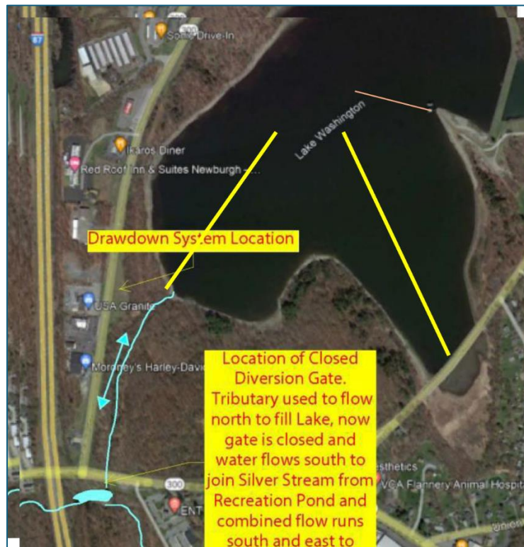
Figure 2. Primary (left) and secondary (right) transects for core sample collection (yellow lines extending from the Lake Washington shoreline). The abandoned wooden trunk line (to be avoided) is indicated in brown.
