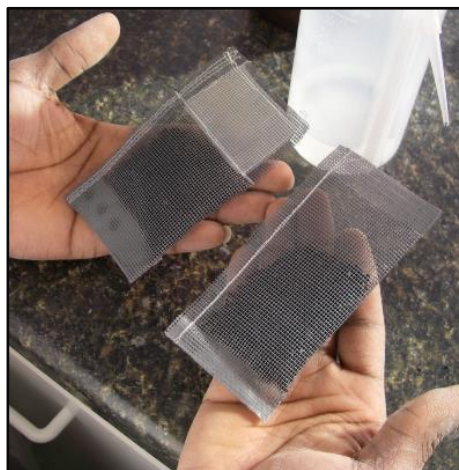
Inset 1: Activated carbon dye samplers.
